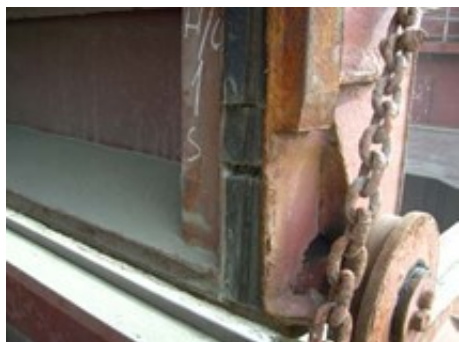
Figure 6: Section replacement of rubber seal
