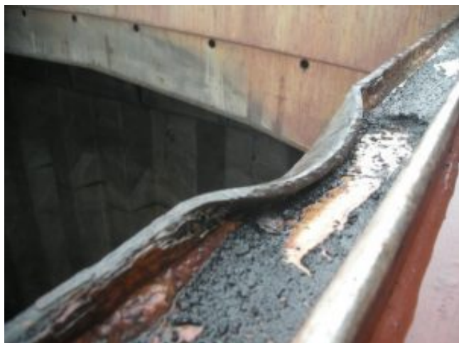
Figure 2: Damaged cargo hatch sill
